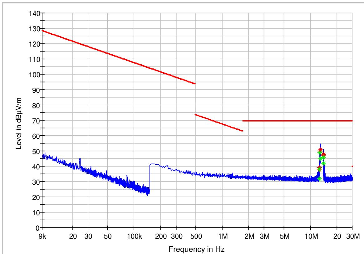
Quasi-Peak detector (< 150 kHz: RBW 200 Hz, >150 kHz: RBW 9 kHz)
