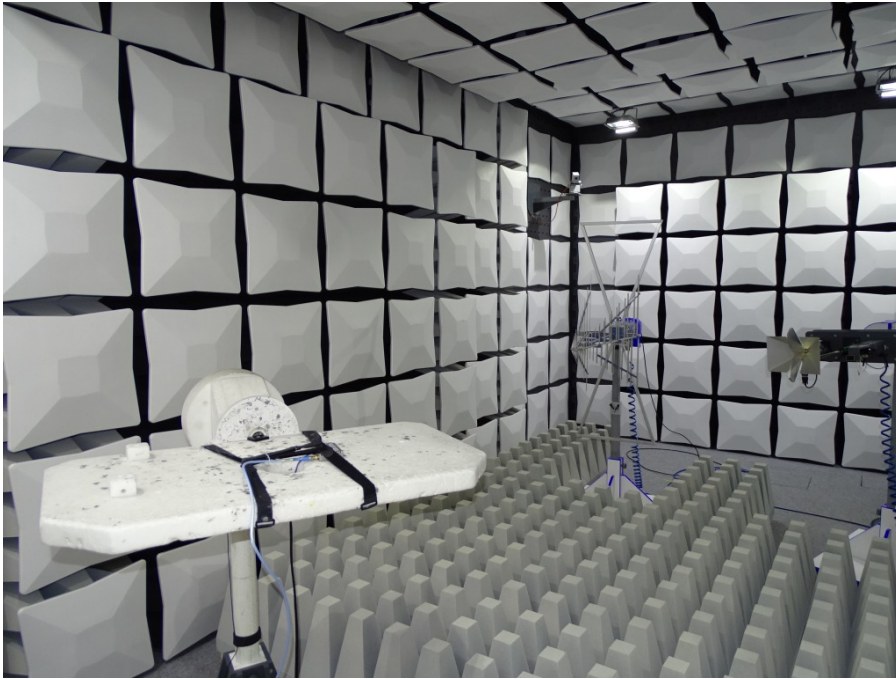
Photo 3: Test setup used for the test case “Radiated spurious emissions” FCC § 20.21 in the range 30 MHz -20 GHz.
