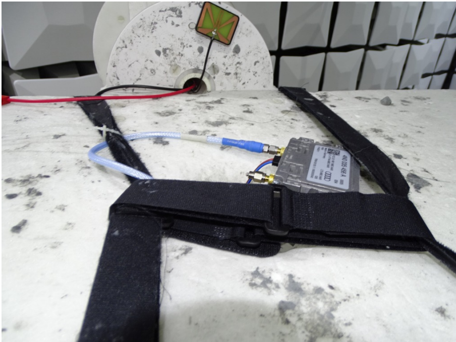
Photo 4: Test setup used for the test case “Radiated spurious emissions” FCC § 20.21 in the range 30 MHz -20 GHz, detailed view.
