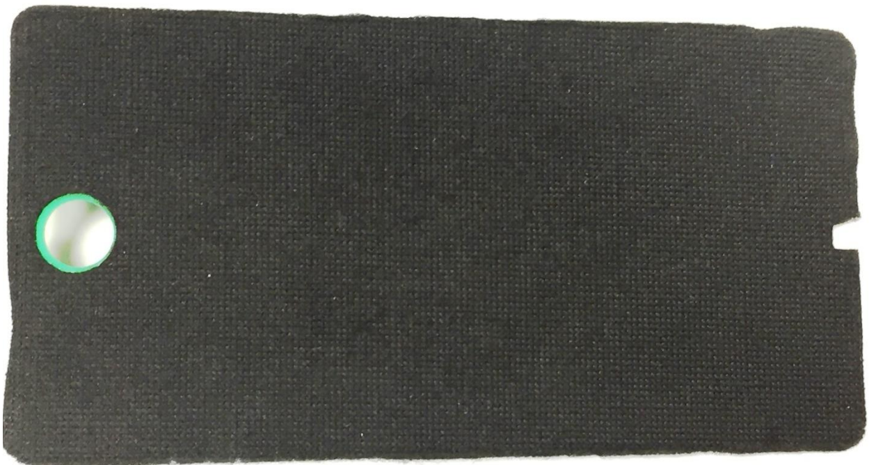
Bottom view of antenna board (Anti-rattle pad glued to it)
