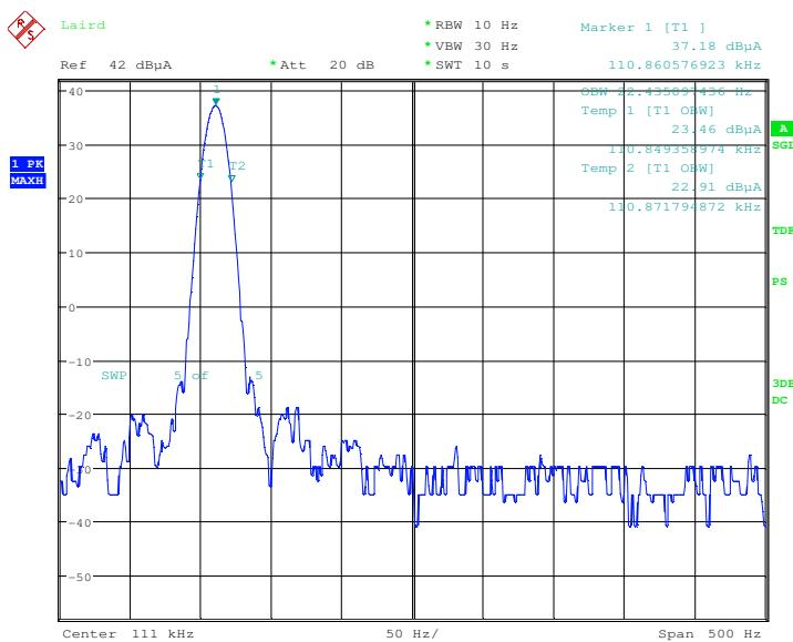
99% Bandwidth / 0.111MHz / WPT\_111kHz\_unmodulated
