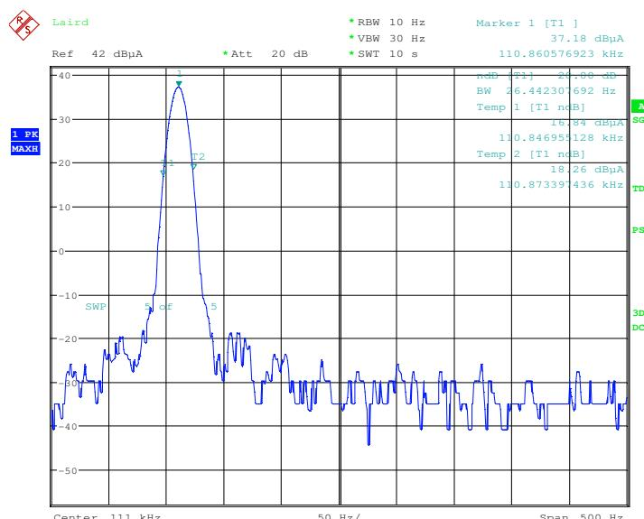
20dB Bandwidth / 0.111MHz / WPT\_111kHz\_unmodulated
