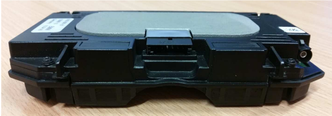
Bottom view (WCH-184c) with System Connector and external antenna connector for Antenna coupler
