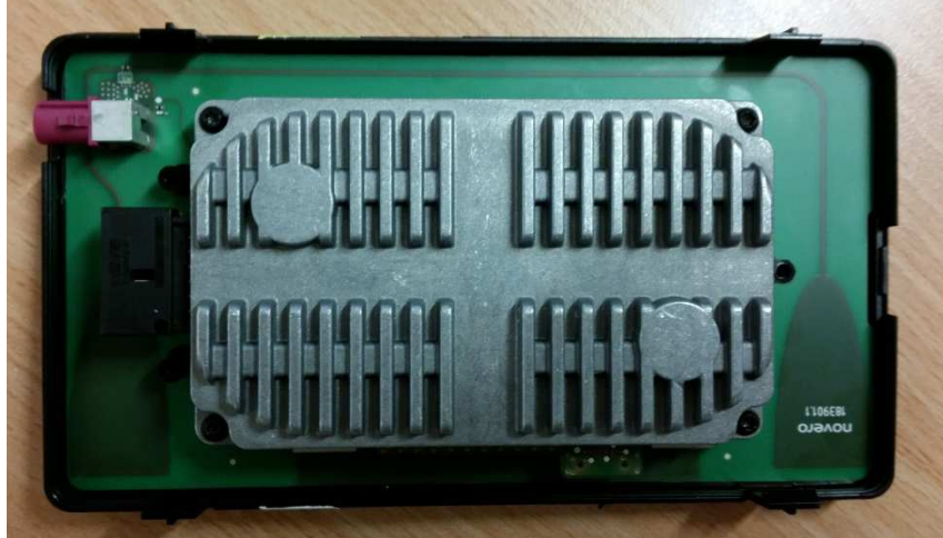
Inside view with PWBs and cooling element
