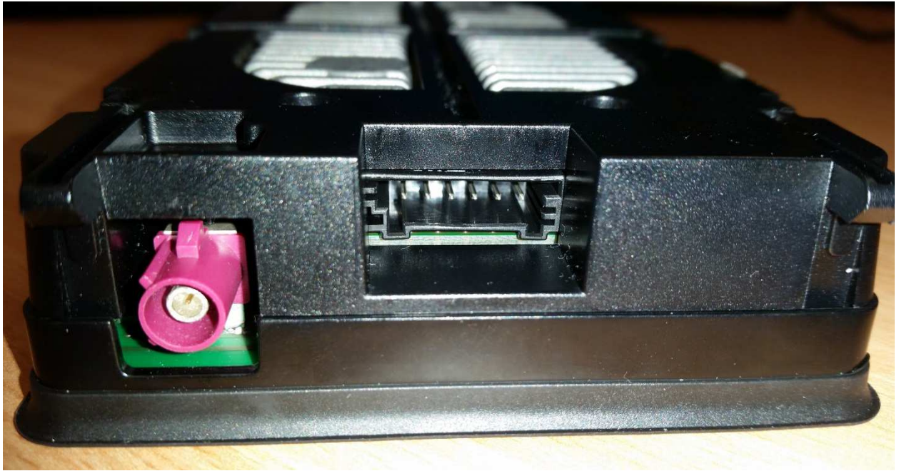
System Connector and external antenna connector for Antenna coupler
