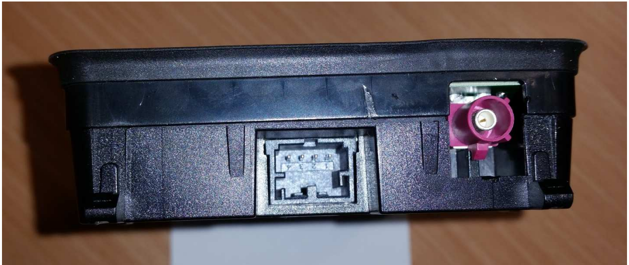
Side view with system connector and external antenna connector for antenna coupler
