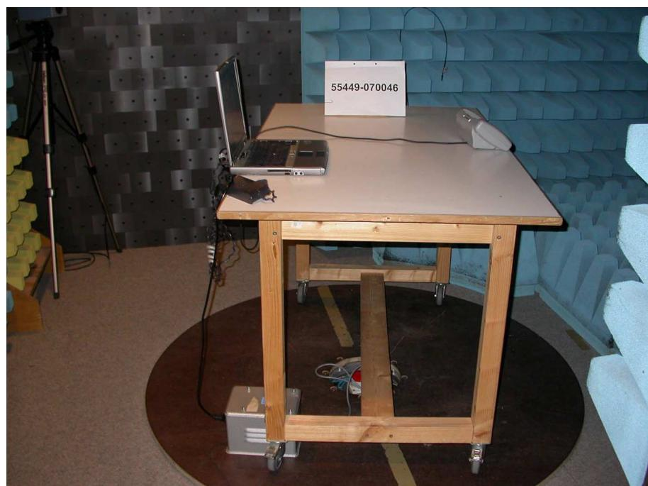
**Test setup for radiated emission measurement
