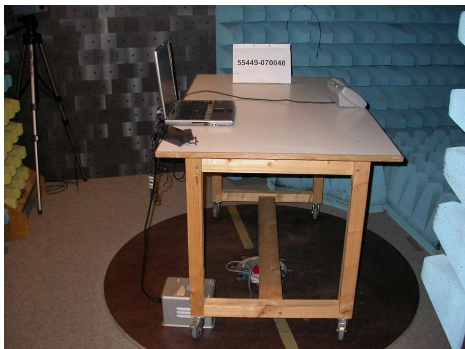
**Test setup for radiated emission measurement
