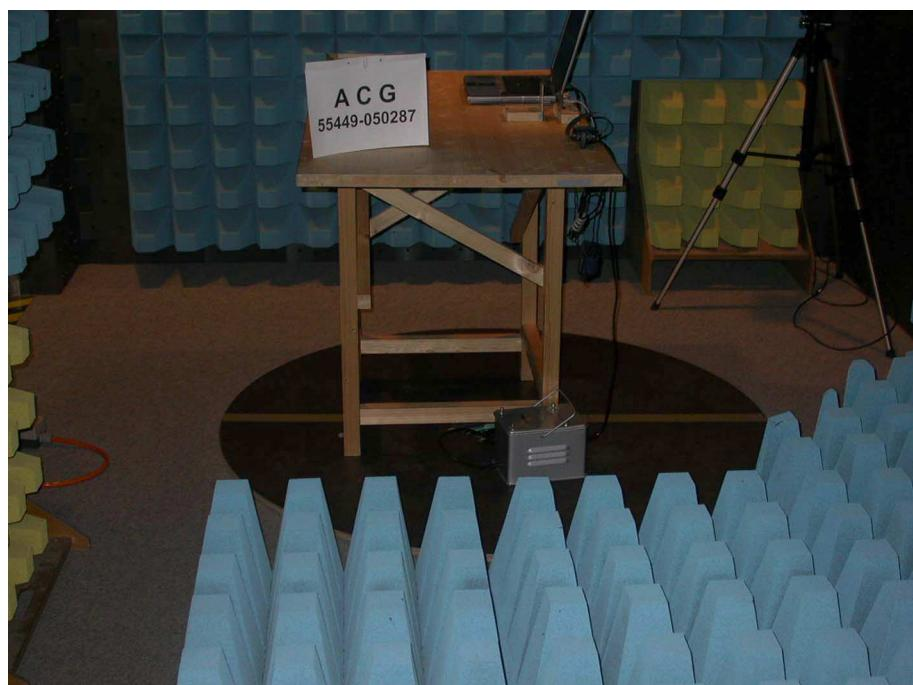
**Test setup for radiated emission measurement
