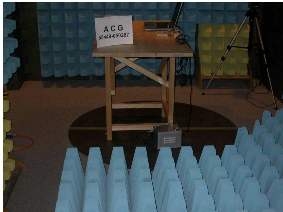
**Test setup for radiated emission measurement
