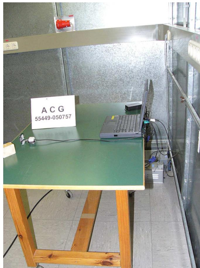
**Test setup for radiated emission measurement 9 kHz – 30 MHz**
