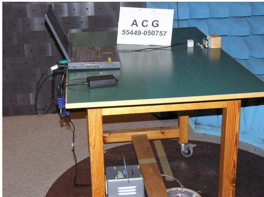
**Test setup for radiated emission measurement
