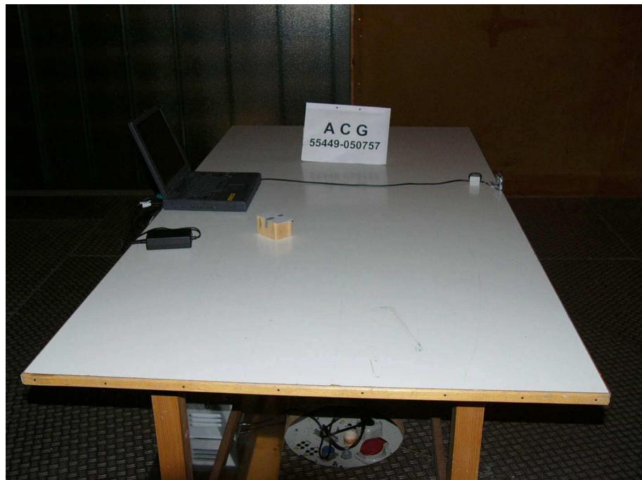
**Test setup for radiated emission measurement
