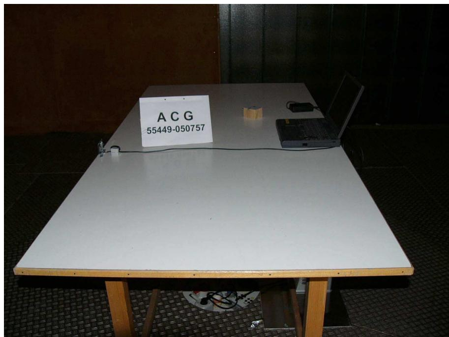
**Test setup for radiated emission measurement
