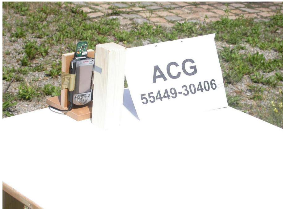
**Test setup for radiated emission measurement
