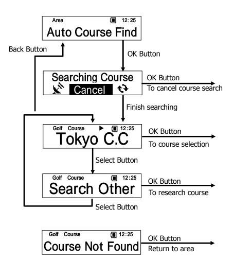
When Auto Course Find is canceled during the search, detected area or prefecture at that point is displayed on the screen. If the area can not be detected at that point, it displays "Out of Area". Refer to 11-3 manual selection for operation in case automatic course selection is canceled during the search.
