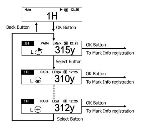
\*The distance to mark will be displayed only if today's Mark Position is received from external device via communication.
