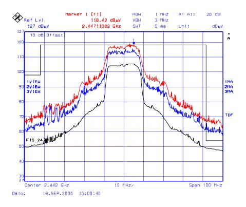
ULTRATECH GROUP OF LABS Fil 3000 Bristol Circle, Oakville, Ontario, Canada L6H 6G4 Tel. #: 905-829-1570, Fax. #: 905-829-8050, Email: <u>vic@ultratech-labs.com</u>, Website: http://www.ultratech-labs.com Plot 29(a): Inner Band-Edge Transmitter Radiated Emissions @ 3 Meters, Horizontal Polarization
