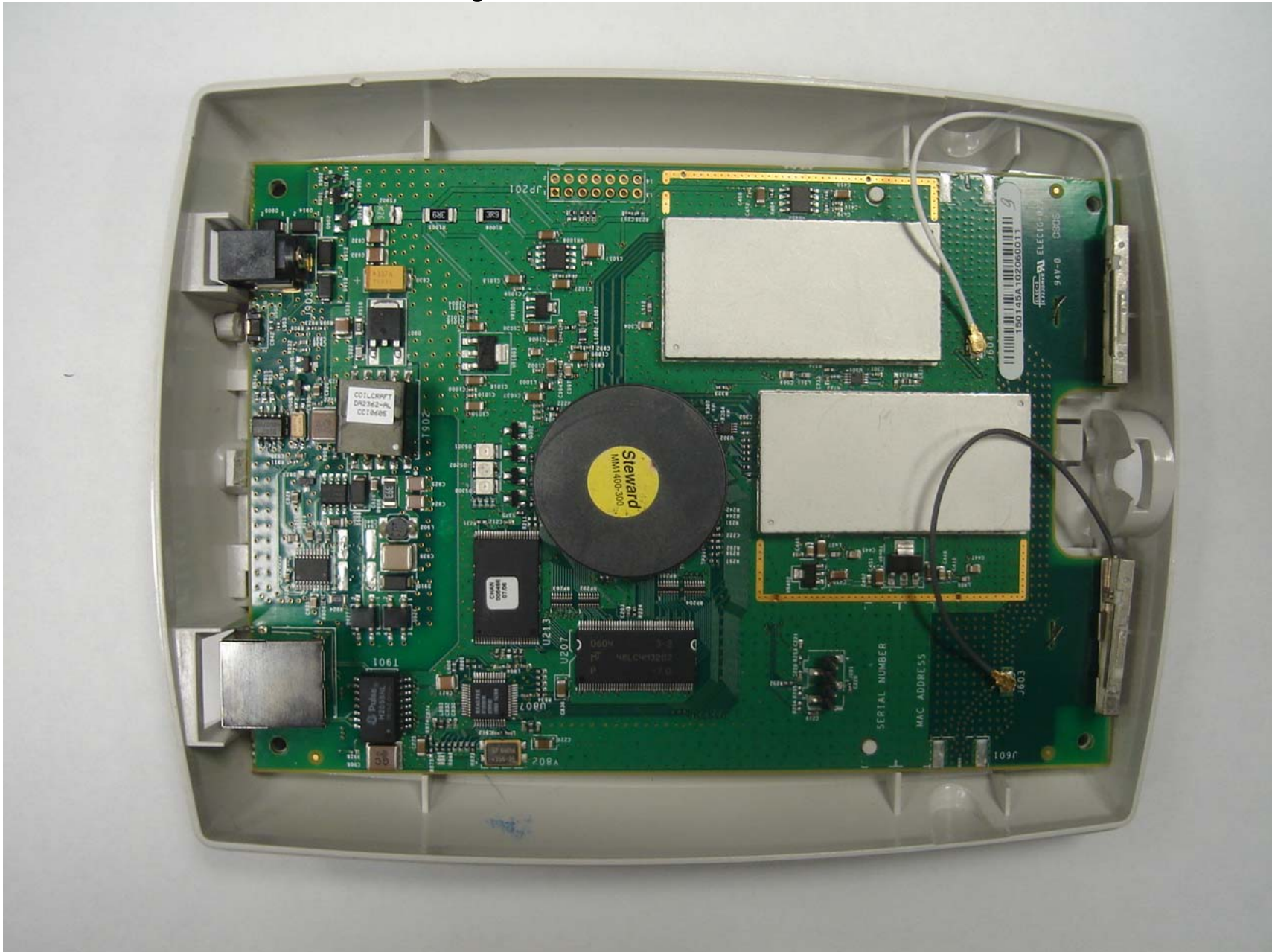
Model Altitude 350-2 Integ 15938 with internal antennas wrt. reversed U.FL connector
