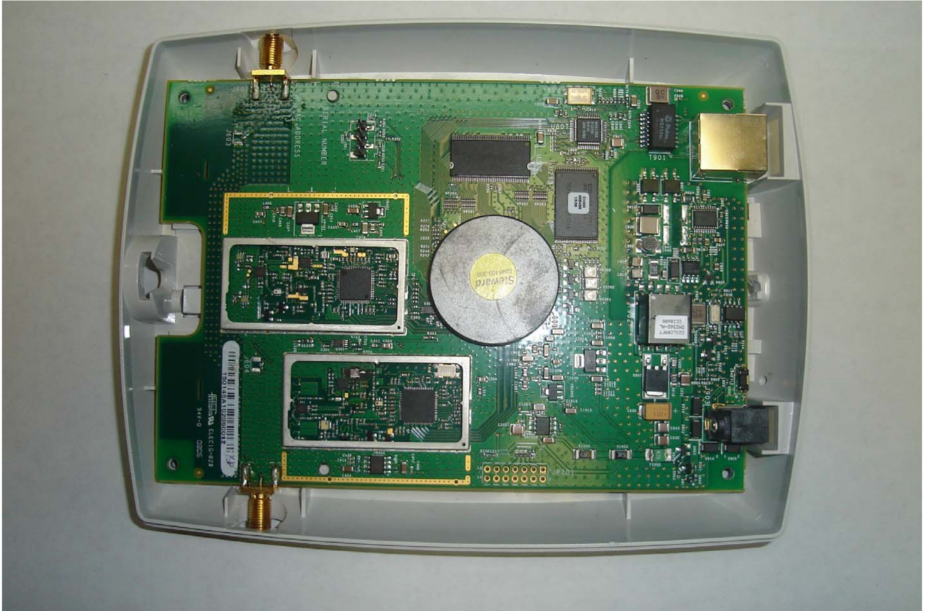
Model ALTITUDE 350-2 DETACH 15939 with external antennas wrt. reversed SMA connector
