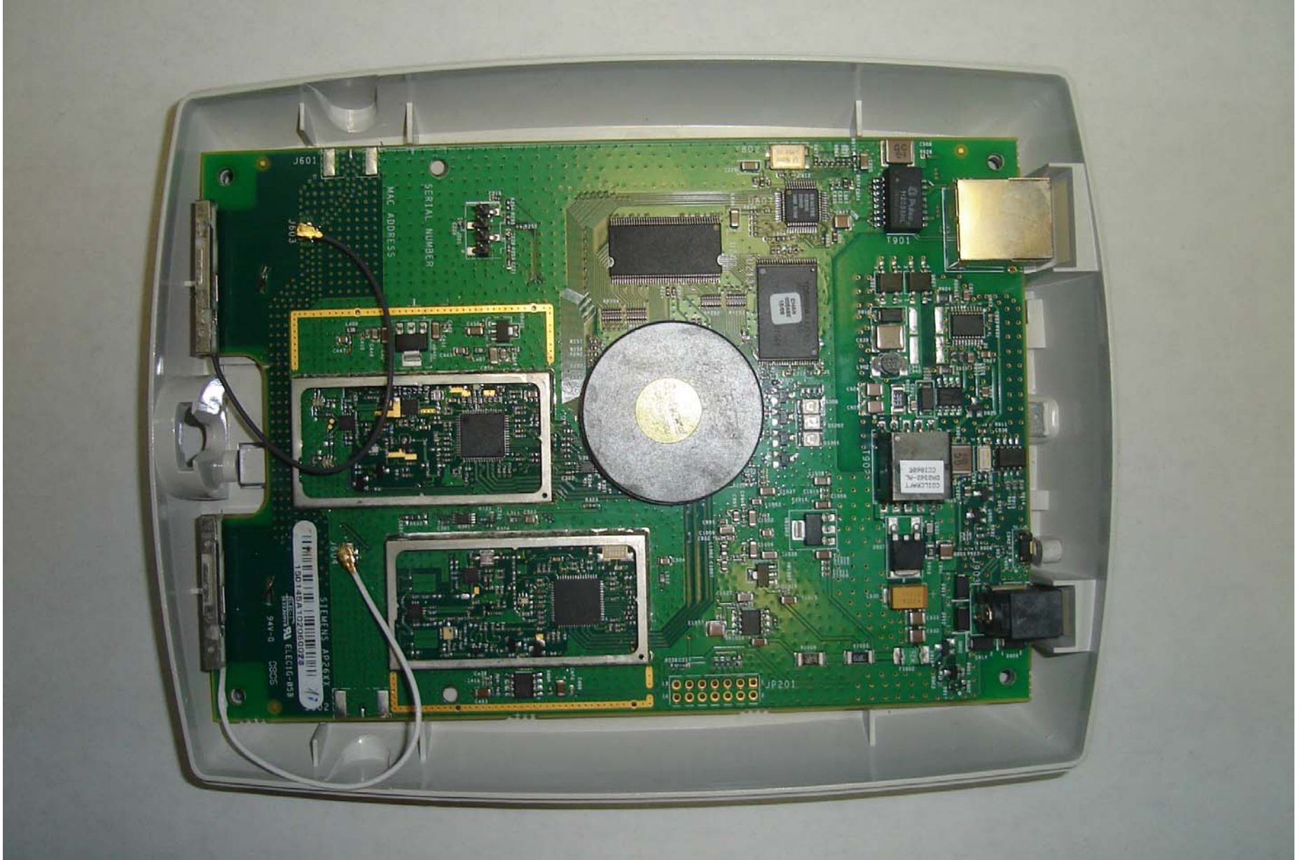
Model Altitude 350-2 Integ 15938 with internal antennas wrt. reversed U.FL connector
