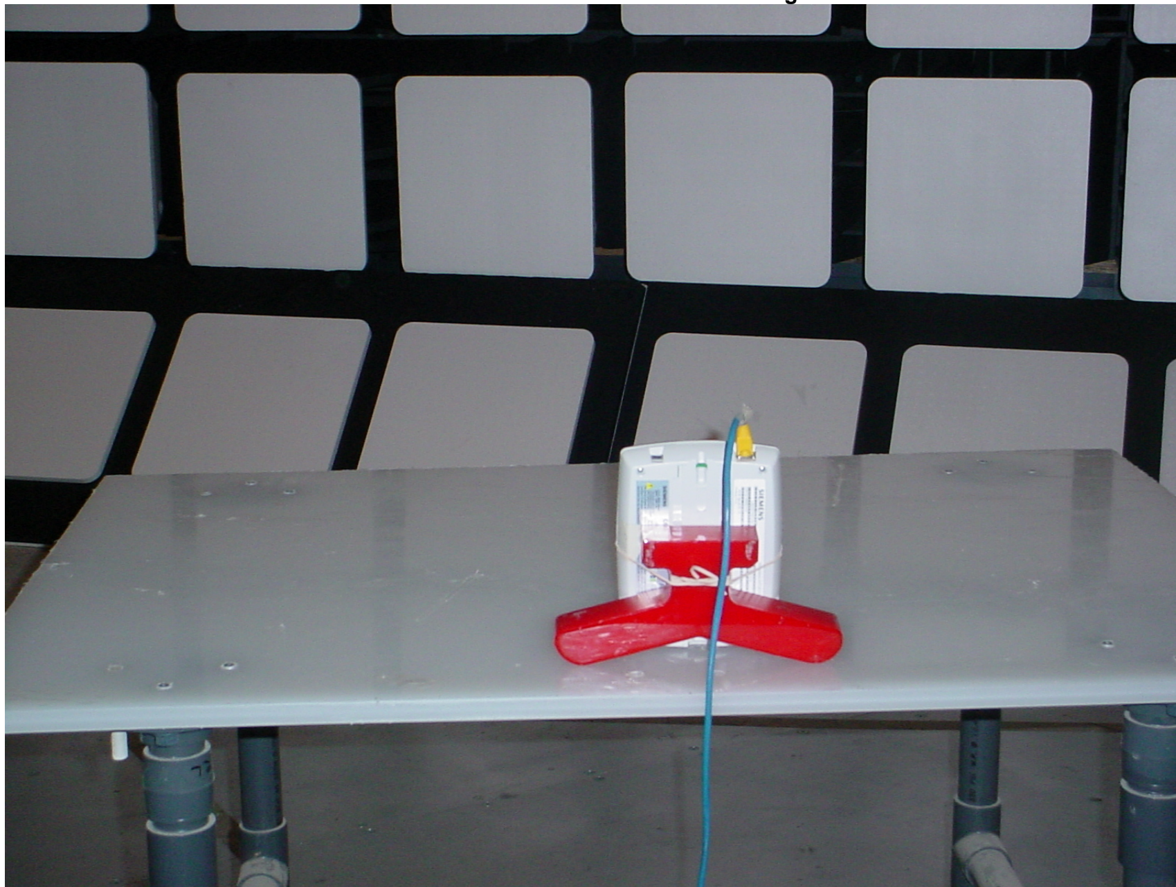
Photo #6: Altitude 350-2 Access Point with external antennas – Test Orthogonal Position #3
