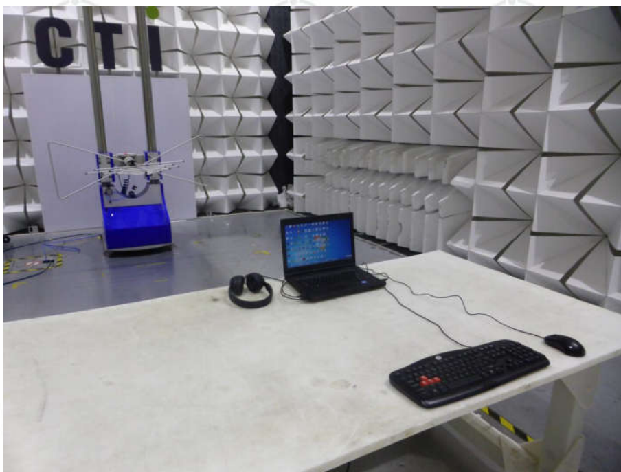
Radiated emission Test Setup-1(Below 1GHz)
