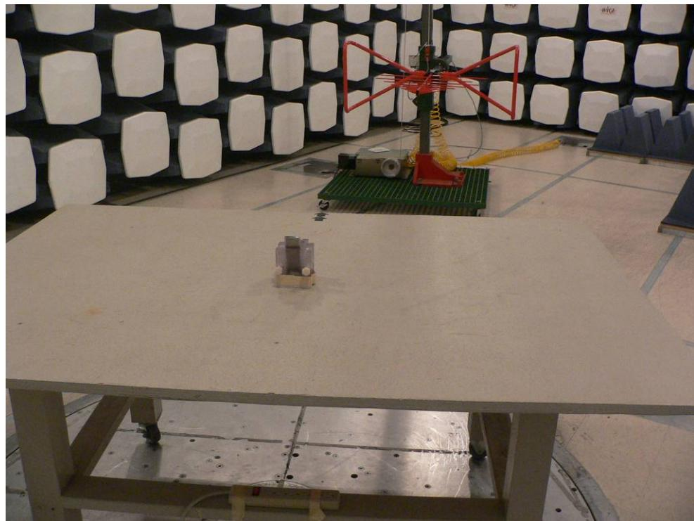
**16.3 Transmitter Radiated Spurious Emissions – Front View**
