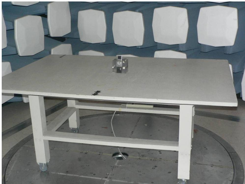
**16.4 Transmitter Radiated Spurious Emissions – Rear View**
