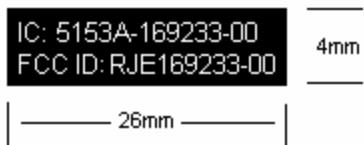
Note1: The Label shall be made of Mylar plastic with adhesive backing
