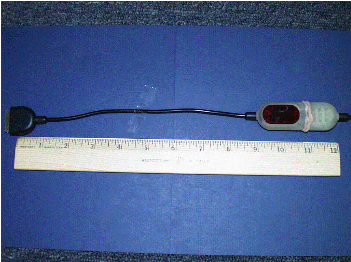
EUT: FM Stereo Full Spectrum Modulator for vehicular use. MODEL : 168007-00 FM Modulator & Antenna
