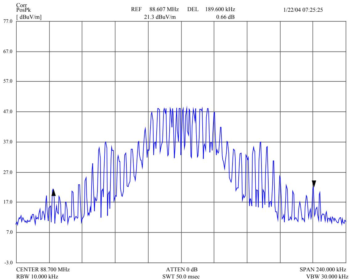
The plot shows the 26 dB bandwidth equals 189.6 kHz
