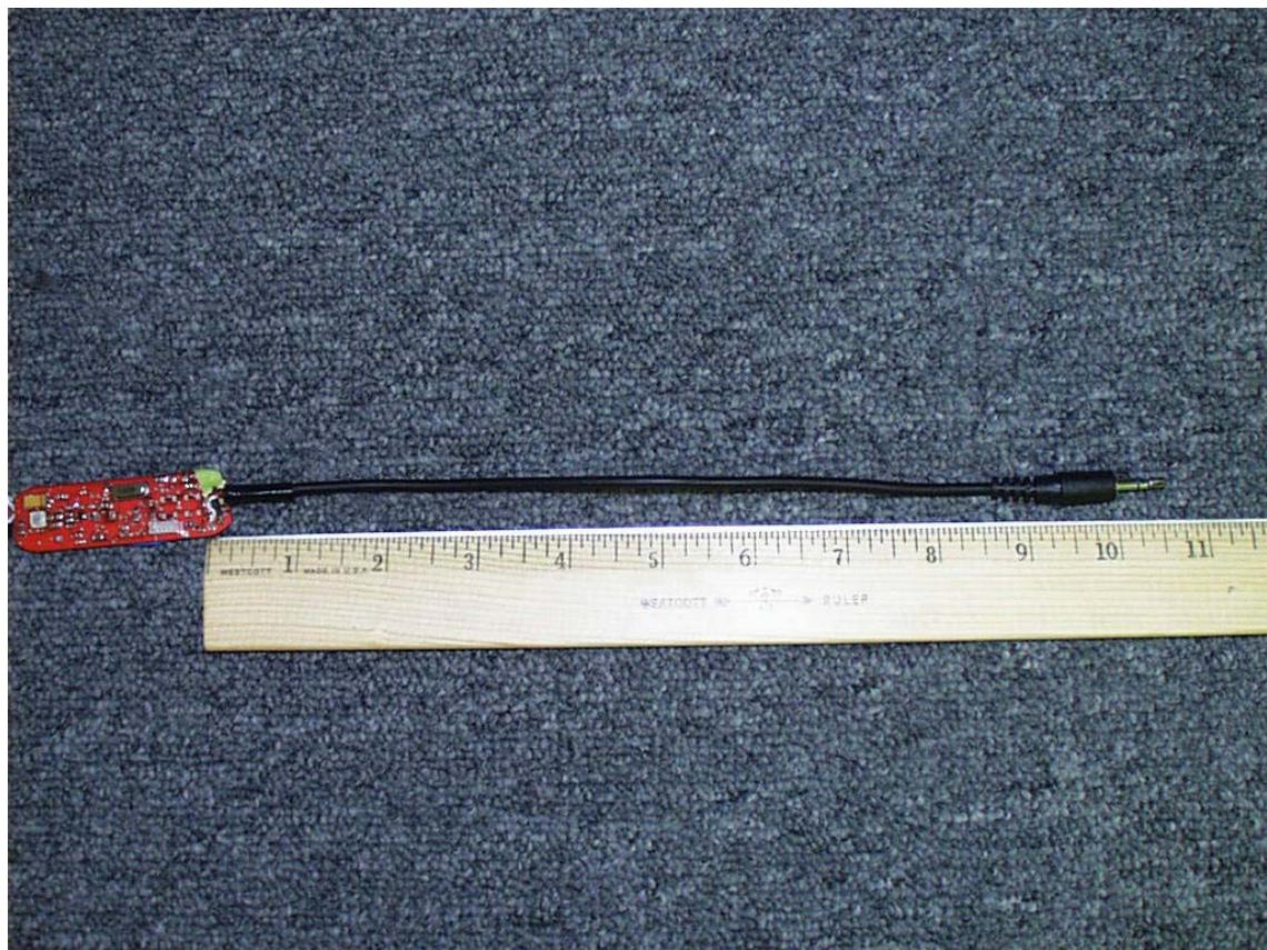
The EUT was configured on a table top. device and was tested with standard MP3 player connected. The modulation frequency was provided by external Test Oscillator HP 651B.
