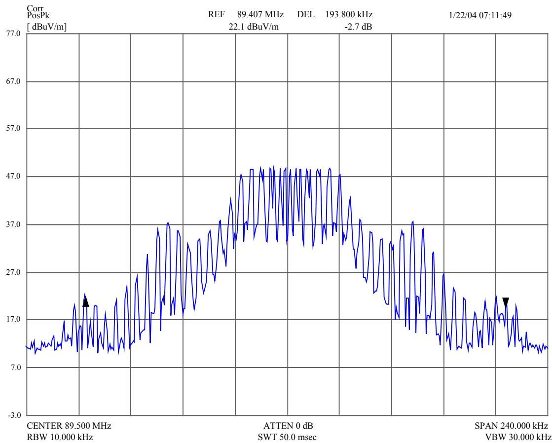
The plot shows the 26 dB bandwidth equals 193.8 kHz
