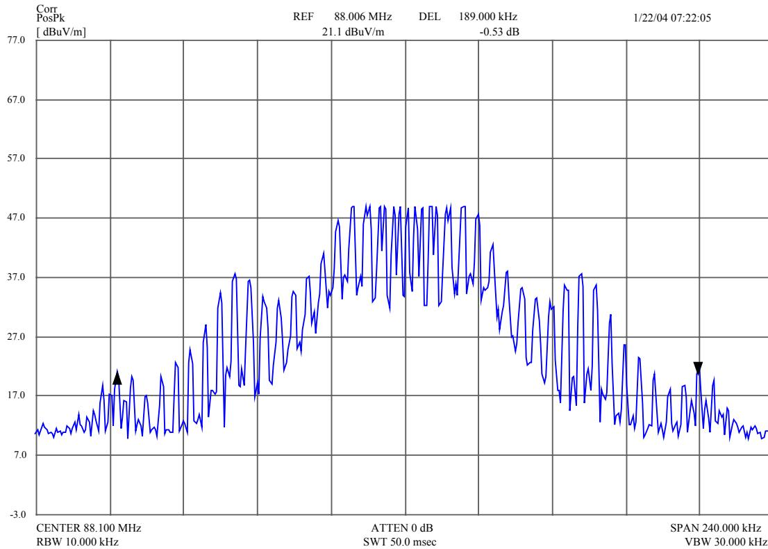
**The plot shows the 26 dB bandwidth equals 189.0 kHz**
