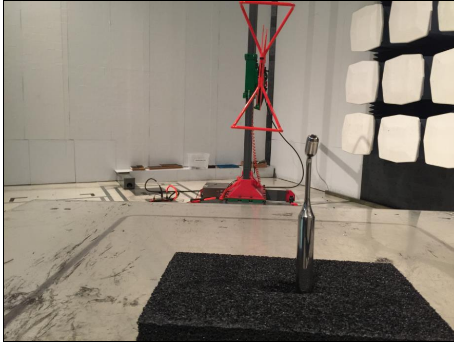
Photograph 1. Radiated Spurious Emissions, Test Setup, Below 1 GHz
