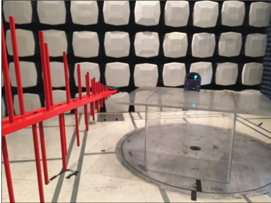
Photograph 1. Radiated Spurious Emissions, Test Setup, Below 1 GHz
