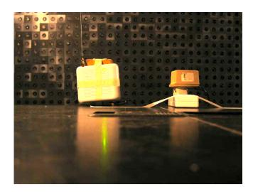
Photograph No.5 Conducted emissions measurement setup
