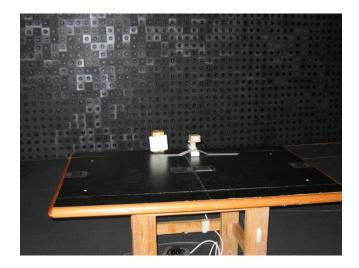
Photograph No.4 Unintentional radiated emissions measurement setup, close view
