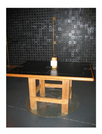
Photograph No.2 Radiated emissions measurement setup in the anechoic chamber, close view
