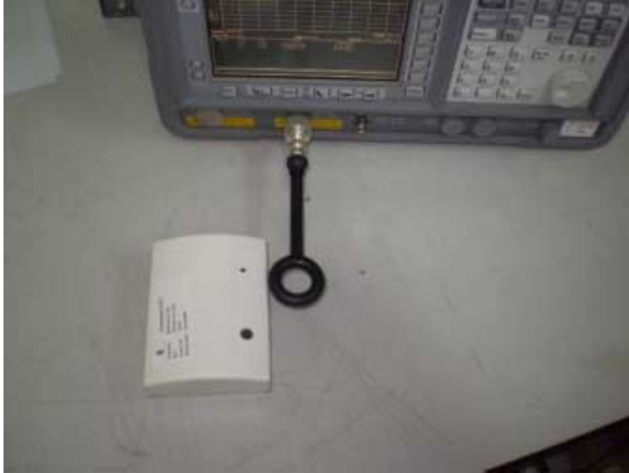
Photograph No.1 Occupied bandwidth measurement setup
