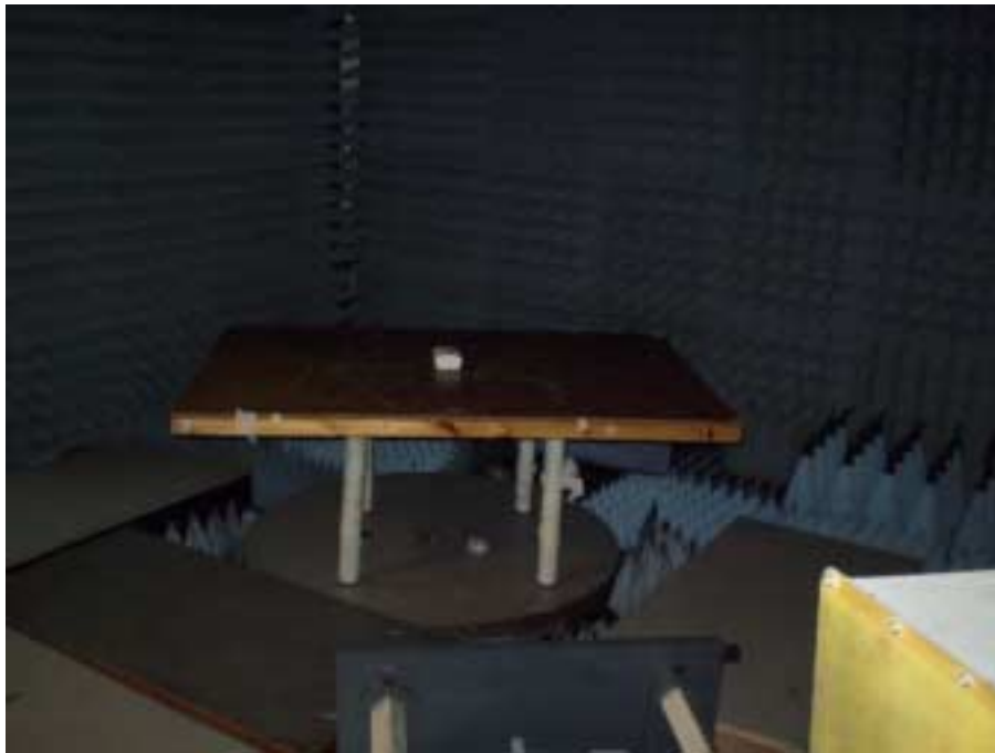
Photograph No.4 Spurious emission field strength measurement setup in the anechoic chamber above 1000 MHz
