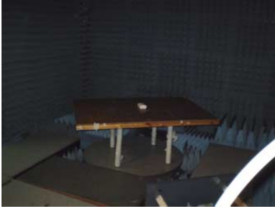
Photograph No.2 Spurious radiated emissions measurement setup in the anechoic chamber in 9 kHz to 30 MHz band
