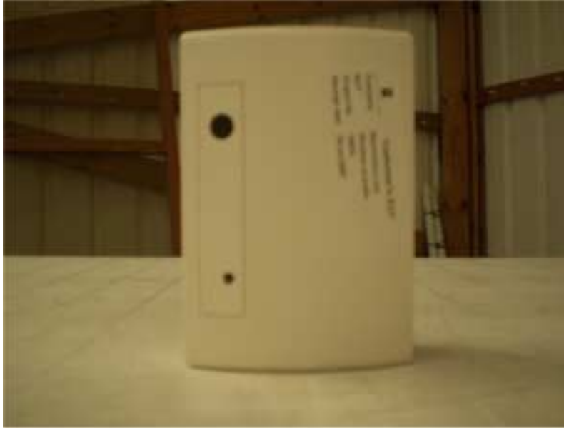
Photograph No.6 Spurious emission field strength measurement setup at the OATS in Y-axis position
