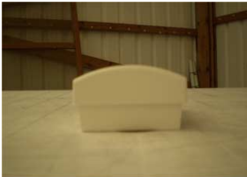
Photograph No.5 Spurious emission field strength measurement setup at the OATS in X-axis position
