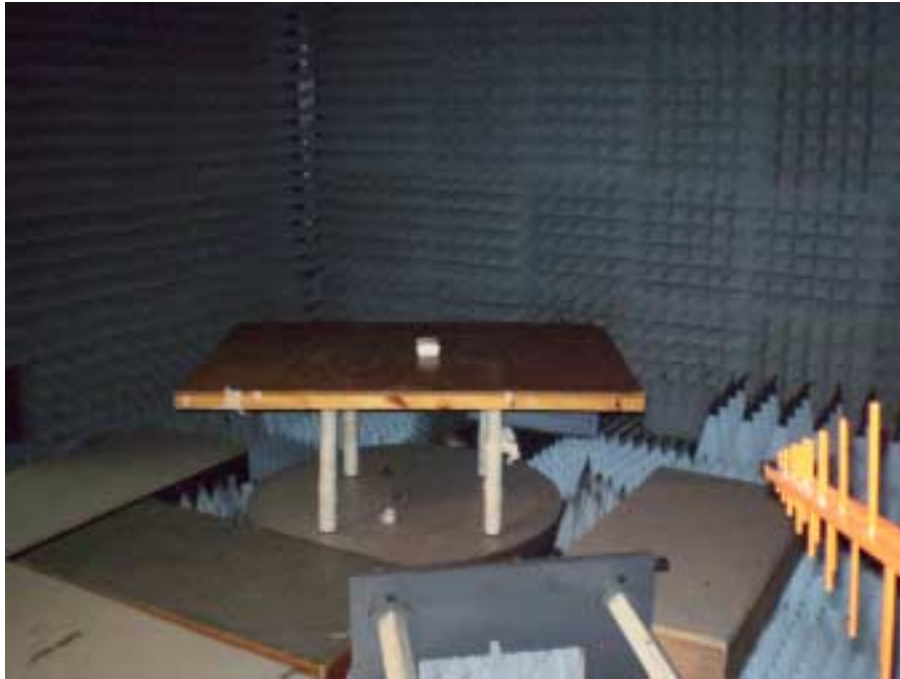
Photograph No.3 Radiated emissions measurement setup in the anechoic chamber in 30 MHz to 1000 MHz band
