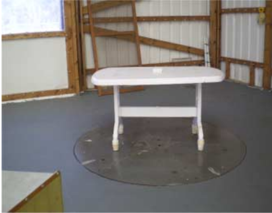
Photograph No.8 Spurious emission field strength measurement setup at the OATS
