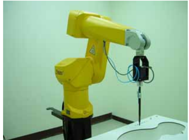
Fig. 5.2 Probe setup on robot
