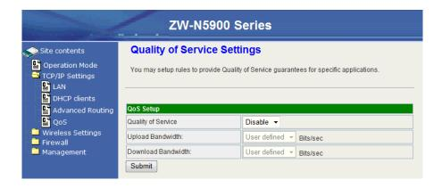
The QoS function is configurable in Gateway and WISP mode.
