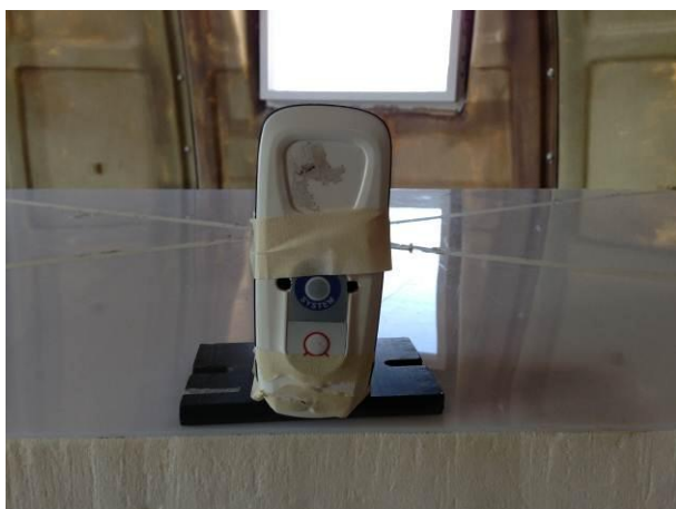
Radiated emission test setup
