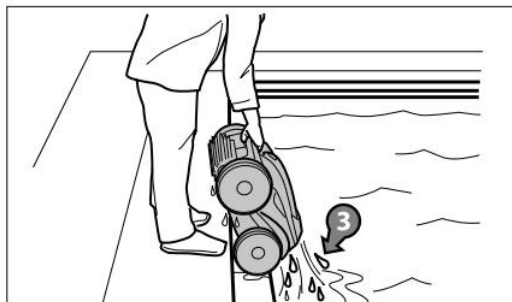
Figure 19. Keep Cleaner Vertical to Drain Water
