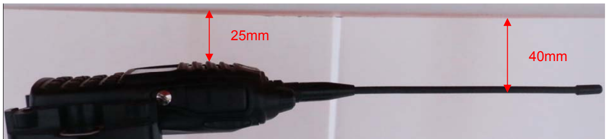
Picture 5: Face-held, the front of the EUT towards phantom, the distance from the EUT Antenna to the bottom of the Phantom is 40mm
