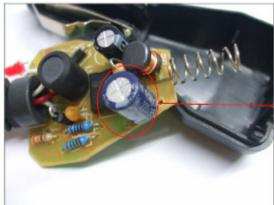
Replace the capacitor with new one which capacitance is 220uF/35V as the picture shown.
