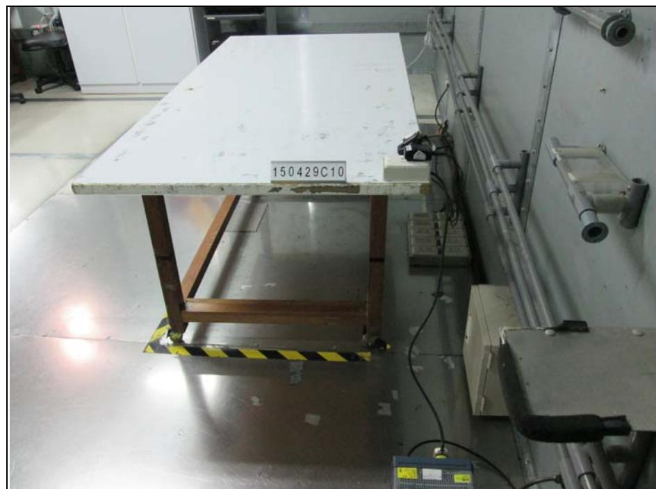
CONDUCTED EMISSION TEST (Test Mode C)
