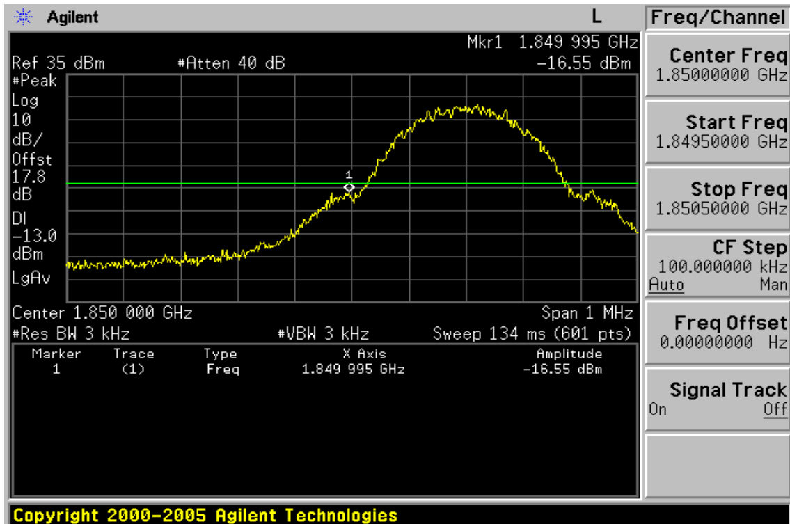
Figure 8-9: Bad edge emission at antenna terminals –PCS 1900 Channel Lowest
