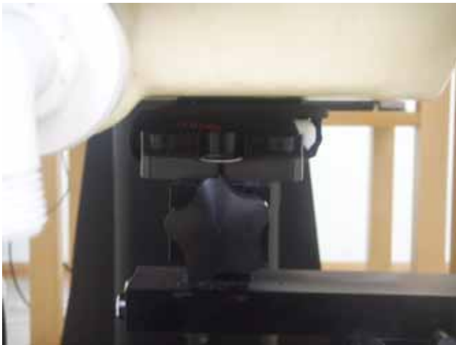
Fig.3 Put the EUT into holster and front side of EUT is paralleled with flat phantom, holster is paralleled and contacted with flat phantom.
