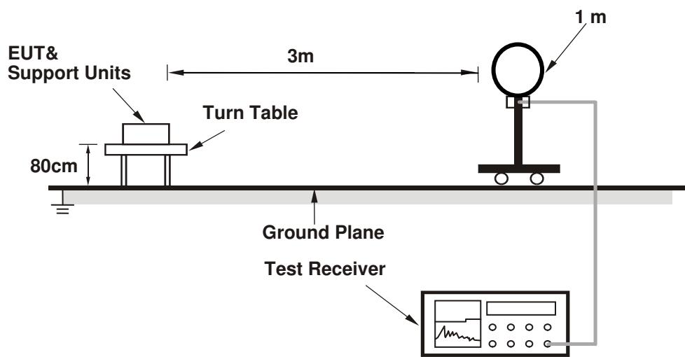
For Radiated emission 30MHz to 1GHz
