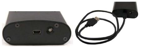
**2.** Plug the USB connector end into an open USB port on the PC with MLOG Controller desktop software loaded (ships with the MLOG Controller).
