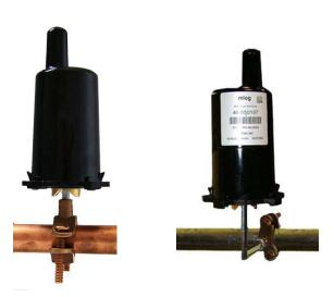
**4.** If the 90-degree angle mounting rod is used, place the pipe clamp as shown (back clamp plate over the screw from the top down for stability) and tighten the screw in an alternating fashion.
