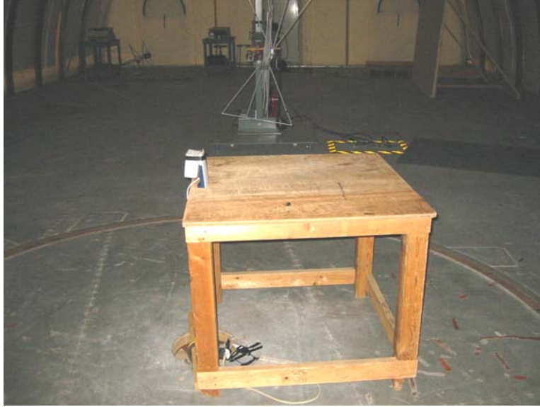
Radiated setup < 1 GHz view 1.
