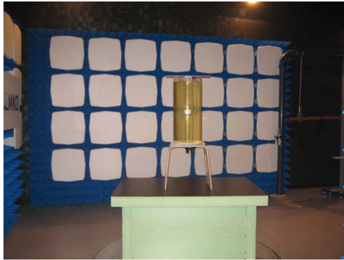
EUT supported 6 cm from torso simulator vertical wall.
