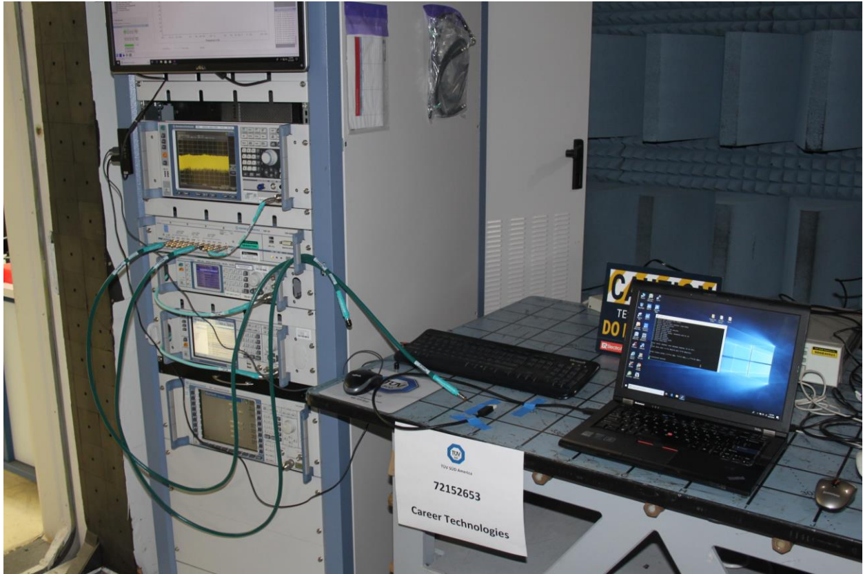
Antenna Conducted Port Test Setup
