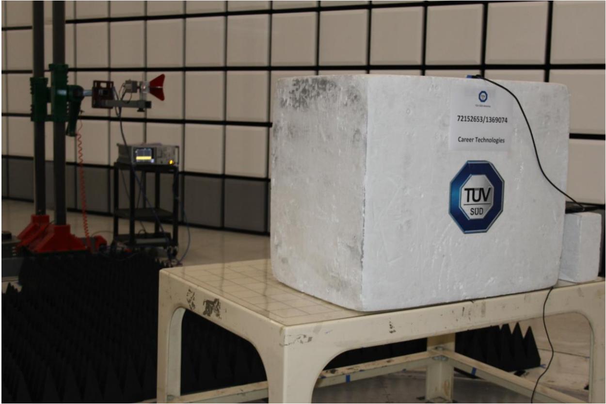
Radiated Emissions Test Setup (above 1GHz)
