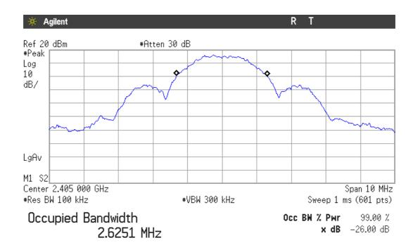
Transmit Freq Error -7.122 kHz x dB Bandwidth 5.106 MHz
