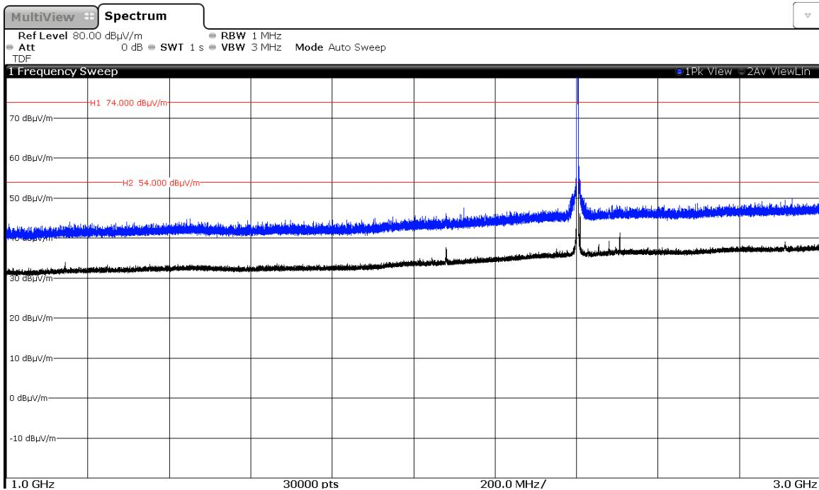
Note: The peak shown in the plot above the limits is the carrier frequency.
