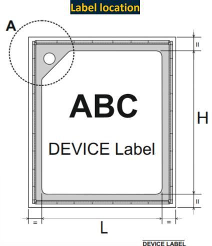
RAW label: 1VV0200872 Dimensions (LxH): 10,7x12,7mm General Tolerance: +/- 0,1mm
