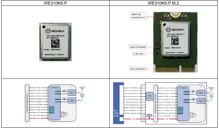
The Main difference is whether the LGA module is mounted on the M.2 interface adapter board.
