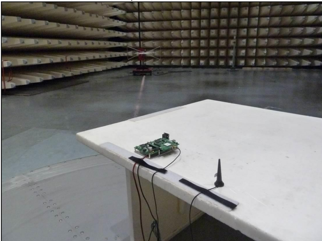
Photo 2: setup of radiated emission < 1 GHz
