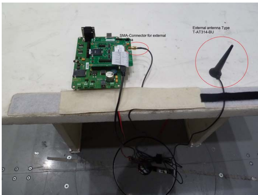
Photo 8 Test system with external antenna:
