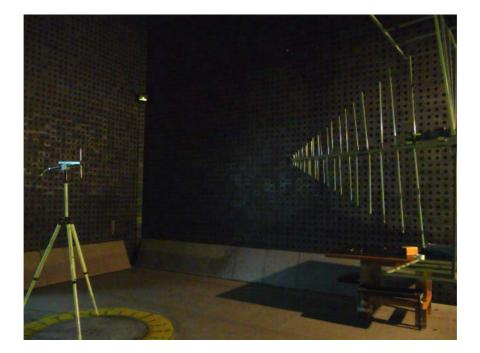
Photograph No.5 Setup for substitution ERP measurements in the anechoic chamber
