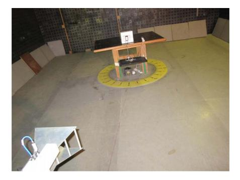
Photograph No.4 Setup for substitution ERP measurements in the anechoic chamber
