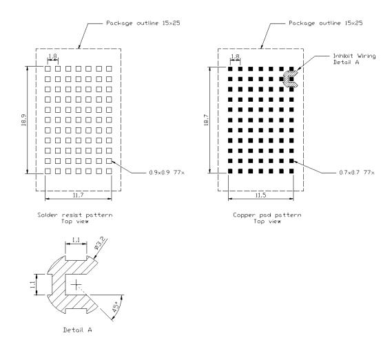
In order to easily rework the UE866 is suggested to consider on the application a 1.5 mm placement inhibit area around the module.
